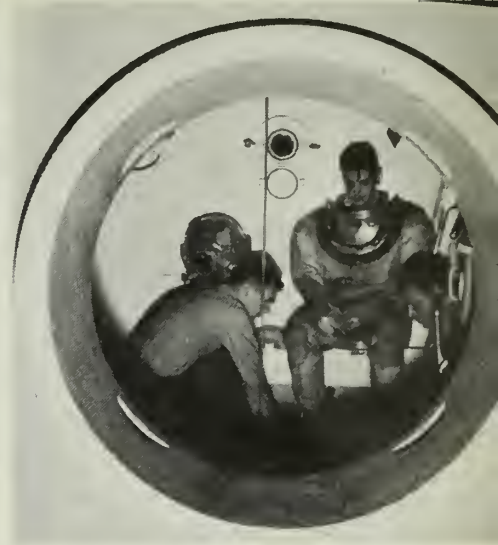
INNER SANCTUM —Theoretical dives in recompression chamber (right) simulate conditions up to 200 and 300 ft. Left: Breast plate is secured to suit.
